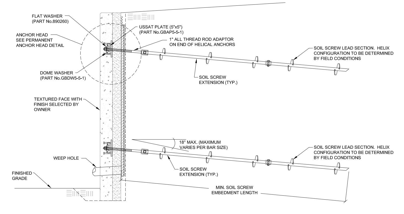
TYPICAL SOIL SCREW CROSS SECTION SHOTCRETE FACING NOT TO SCALE
