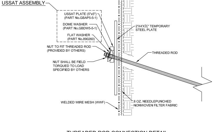
THREADED ROD CONNECTION DETAIL WITH TEMPORARY FACING NOT TO SCALE
